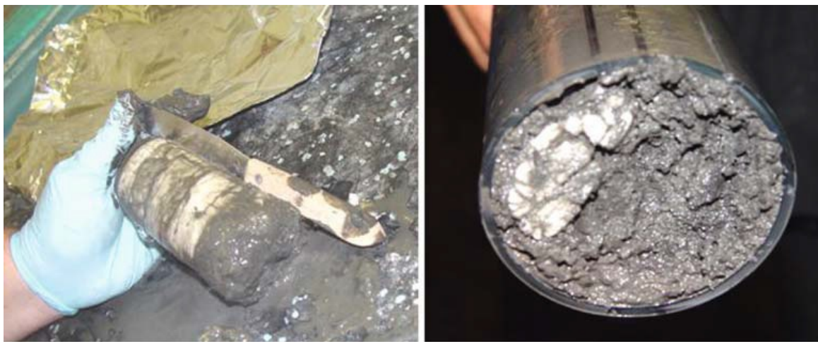
Figure.5. Massive and disseminated form of gas hydrate recovered from KG offshore during NGHP expedition (Source: Ramana & Ramprasad, 2010)
