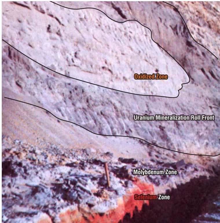
Figure 5 – Pit wall cross section of uranium roll-front (bio-geochemical cell) (After Dickinson and Duval, 1977)
