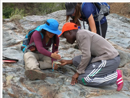
Alejandra Santiago Torres, Lois Kamuyango and Amy Pritt measure the orientation of foliation in Precambrian gneiss near
