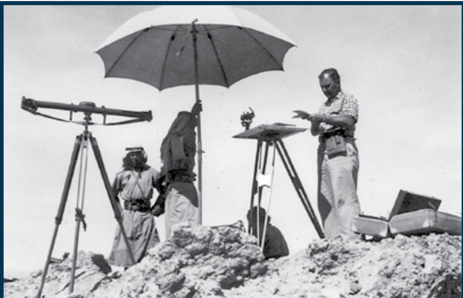
René Wetzel (right) with a guard, range finder and plane table. Photo courtesy of D.M. Morton.
