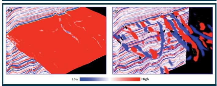
Figure 3 – Vertical slice of seismic amplitude and stratal slices through (a) seismic amplitude and (b) a merging of coherence (black), most-positive principal curvature (red), and principal most-negative principal curvature (blue) volumes. Transparency has been used to retain only very low coherence values, very high positive curvature and very low negative curvature.
