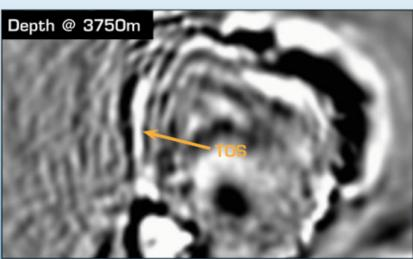
Same depth slice after Dual Flood RTM. Prism waves image the salt flank, giving an accurate geometry to the mini basin.
