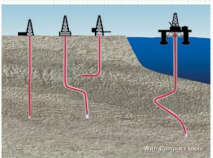
Compact formation evaluation (FE) tools are half the size of most conventional wireline equipment and offer eleven different conveyance options. So now you can gain access to more hole sizes and log problematic wells with less risk of getting stuck.
