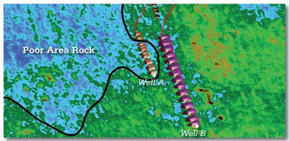
Here, results show that stimulation programs can be optimized based on rock properties from seismic.
