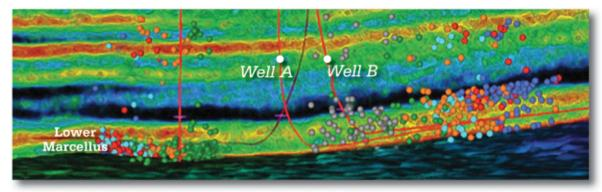
Thickness of the ductile layer above the Lower Marcellus (blue) influences the degree to which fracs remain constrained.
