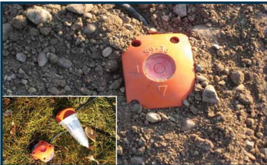
The 3-component geophones used to record the Vector Bakken 2-D/3C test line are true geophones. Each phone was buried in a pre-drilled pilot hole.
