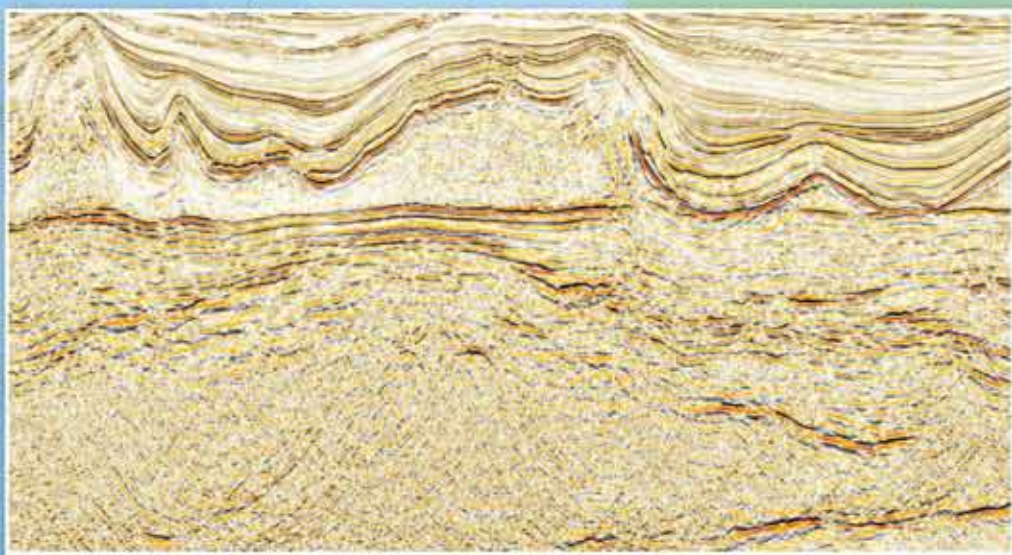
Intermediate prestack depth migration: salt flood, anisotropic tilted transverse isotropy (TTI) adaptive beam.
