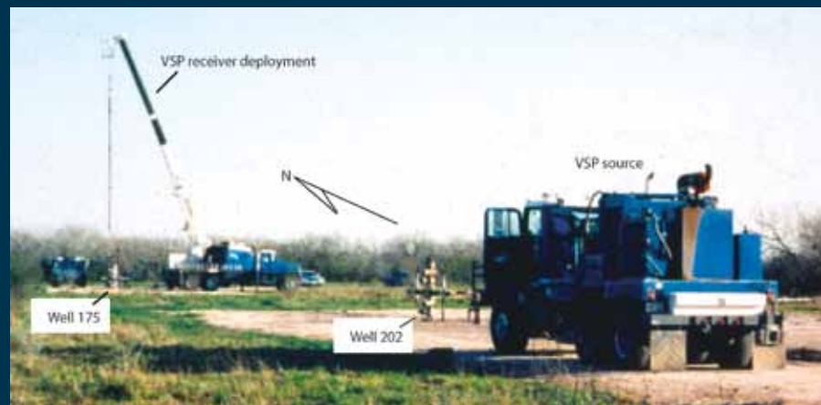
Figure 4 – Photo showing the proximity of wells 175 and 202. It is sobering to think a reservoir compartment boundary occurs in the short interwell distance between these two wells. In this photo, a zero-offset VSP is being acquired in well 175. For the data shown on figure 3, the receiver system was in well 202 and the vibrator source was far to the north of well 175.
