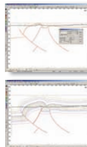
Figures 1&2: Original horizon and reconstructed fold using the construct beds toolbox in 2DMove™.
