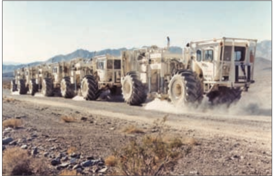
A whole lotta' (test) shaking going on: Specialized trucks vibrate the ground to simulate natural seismic activity at Yucca Mountain.
