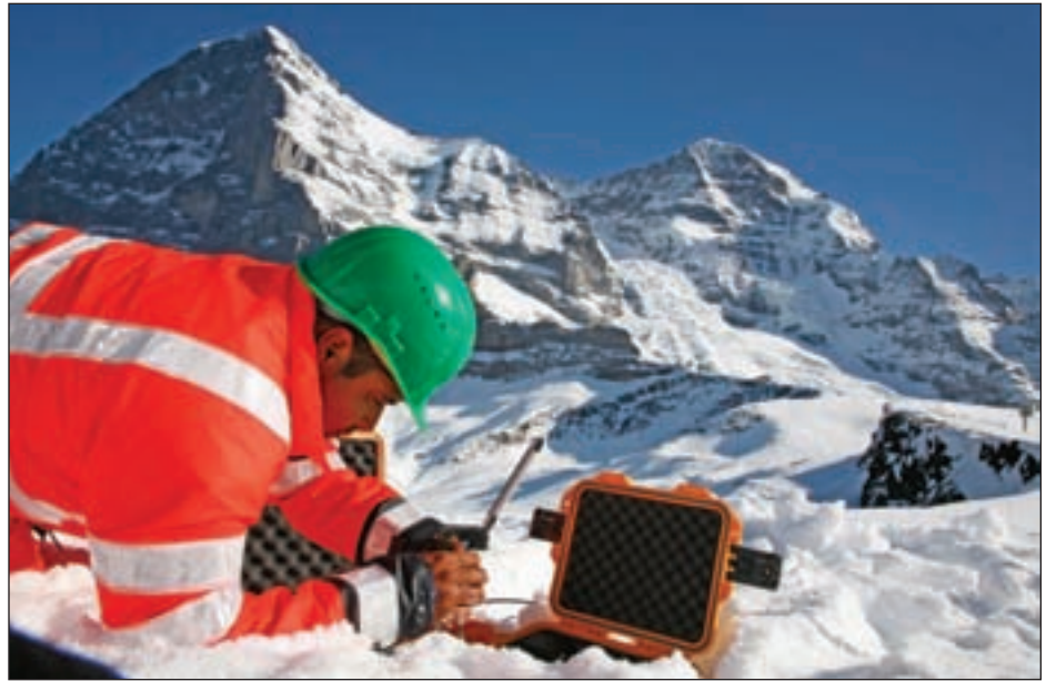
Do not disturb (the surroundings): A technician tests broadband receiver stations, demonstrating passive seismic operations, in the Swiss Alps.
