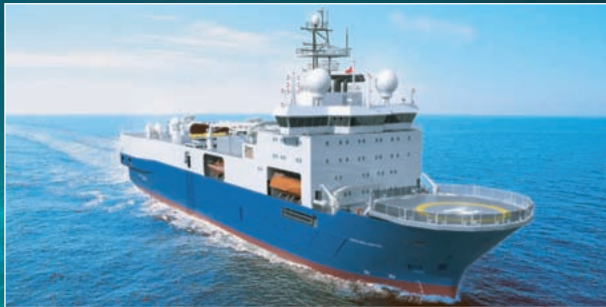
Geo Atlantic - New 2006! Maximum streamer capacity 10 x 8 km.
