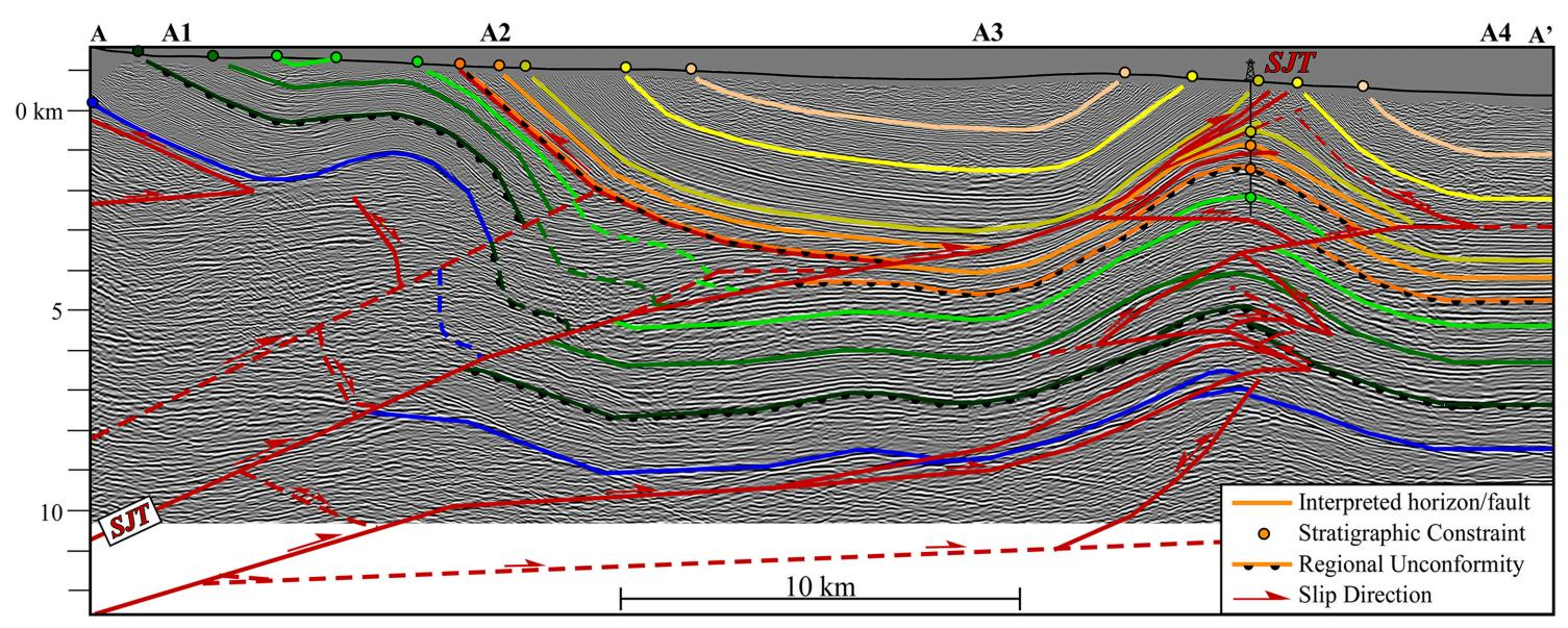
Figure S1. Seismic interpretation of section AA'. See text for details. Stratigraphy is constrained by surface geology, well data, and our regional seismic interpretations. Uninterpreted section is shown in Figure 4A. See Figures 1 and 2 for section location.
