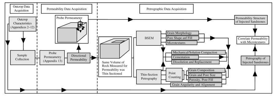
**Appendix 1.** Workflow from outcrop to permeability and petrographic data acquisition. BSEM = backscattered-electron microscopy.
