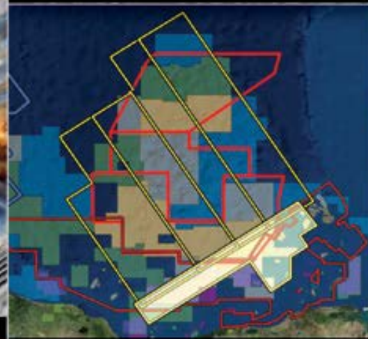
Acquisition of long-offset broadband WAZ seismic data covering 9,900 km² of Campeche shallow water will be completed ahead of the Round 2.1 lease sale.
