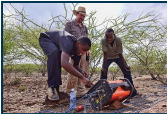
Volunteer geophysicist Randy Shundike and Katila and Odonga, students in IsraAID's WASH program, run the ABEM LS system for resistivity imaging near Kaolobeyei. Photo courtesy of GWB.
