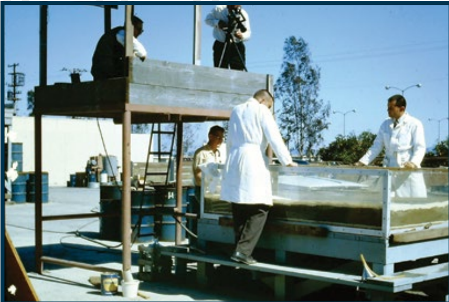
January Manley Natland (with camera) filming the generation of turbidites in a flume at Union Oil Research Laboratory, Brea, Calif., January 1965. Photo courtesy of Martin Natland.
