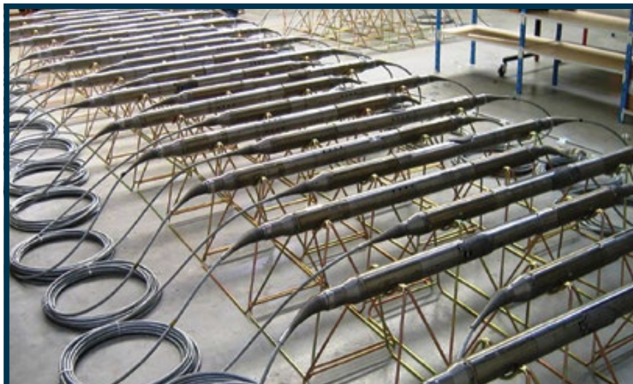
Sercel's Geowave II was the industry's first digital multi-level array specifically designed for high-temperature, high-pressure wells.
