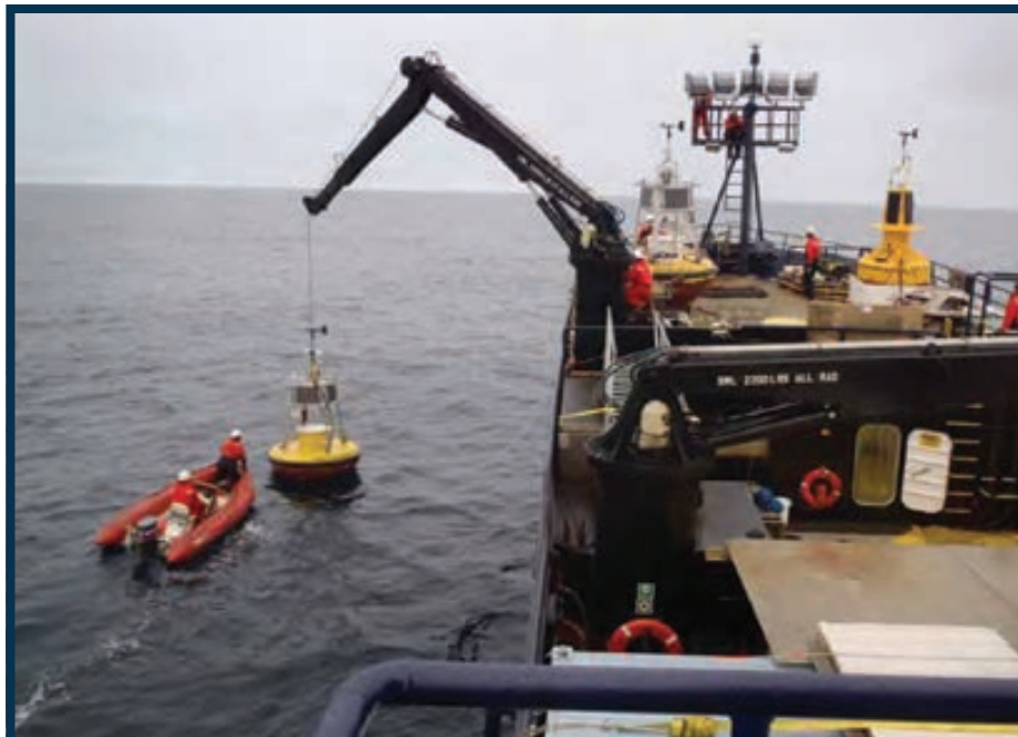
The vessel crew deploys a metocean buoy from the westward wind.
