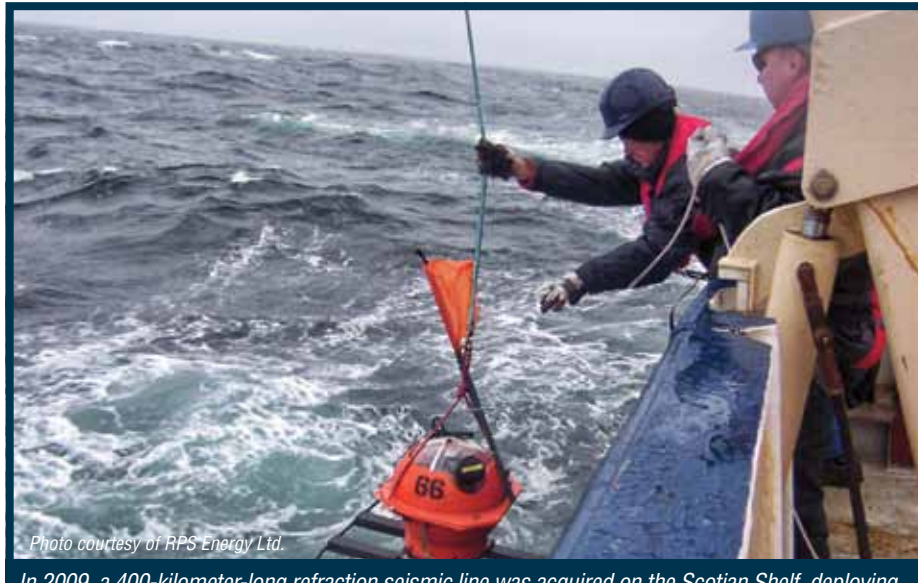
In 2009, a 400-kilometer-long refraction seismic line was acquired on the Scotian Shelf, deploying 100 three-component ocean bottom seismometers (OBSs), shown above.
