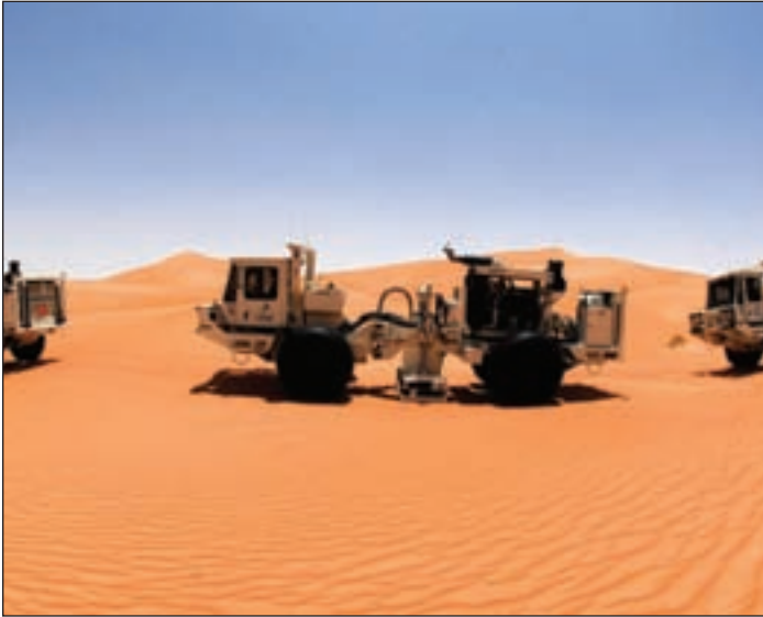
Headed for international duty: The 60-foot Global Quest (left) was transported to India for a challenging shallow marine program in the Gulf of Khambhat; the 60,000 pound vibrators spent their time in Algeria.
