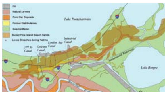
Depositional Environments of Lower Mississippi River Deltaic Plain - New Orleans Metro Area.
